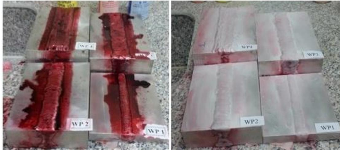
**penetrant testing of the welded joints from front sides
