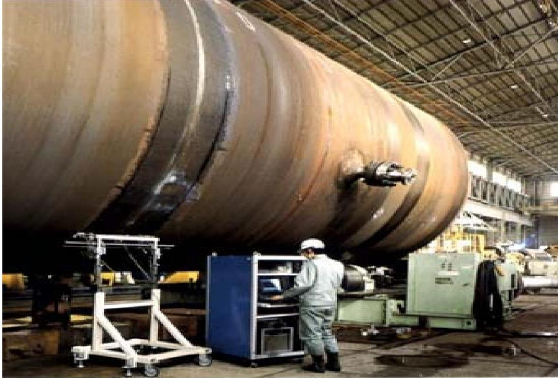
Fig. 8 TOFD being done for a heavy walled pressure vessel at shop <sup>[5]</sup>
